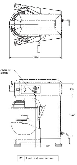
MACHINE ELECTRICAL SPECS: 120/60/1 – ETL Listed
