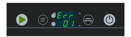
▶ The error code is shown in the bottom display (see table).
